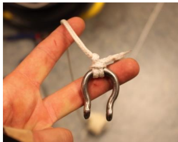
Figur 7- A clove hitch is used to fasten the CTD to the winch rope.
