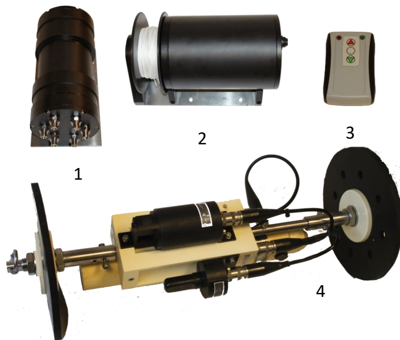
Figur 3 - Main parts. 1. Main controller, 2. Winch, 3. Remote, 4. Mutiparameter CTD with protection kit
