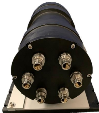
Figur 13- Main controller/Unit el-tube w/6 different pins number.
