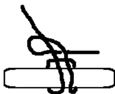
Figur 7- A clove hitch is used to fasten the CTD to the winch rope.
